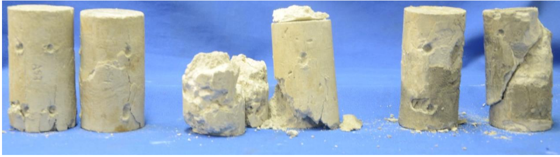
Figure 7.15 Two-component grout specimens after being tested
