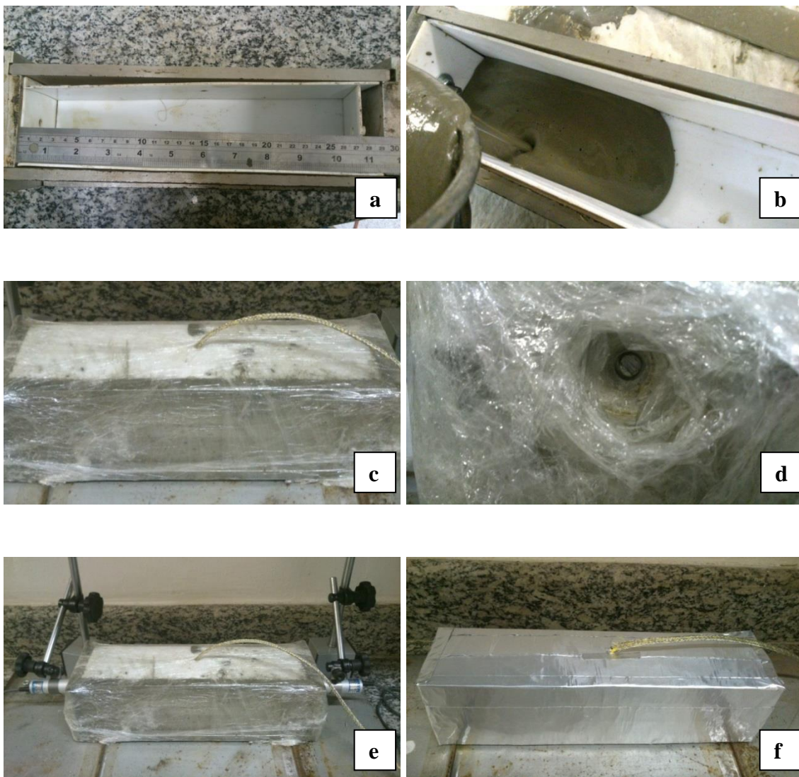
Figure 4.23 Autogenous Shrinkage test procedure
