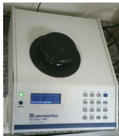
Figure 4.11 Gas pycnometer used for experiments
