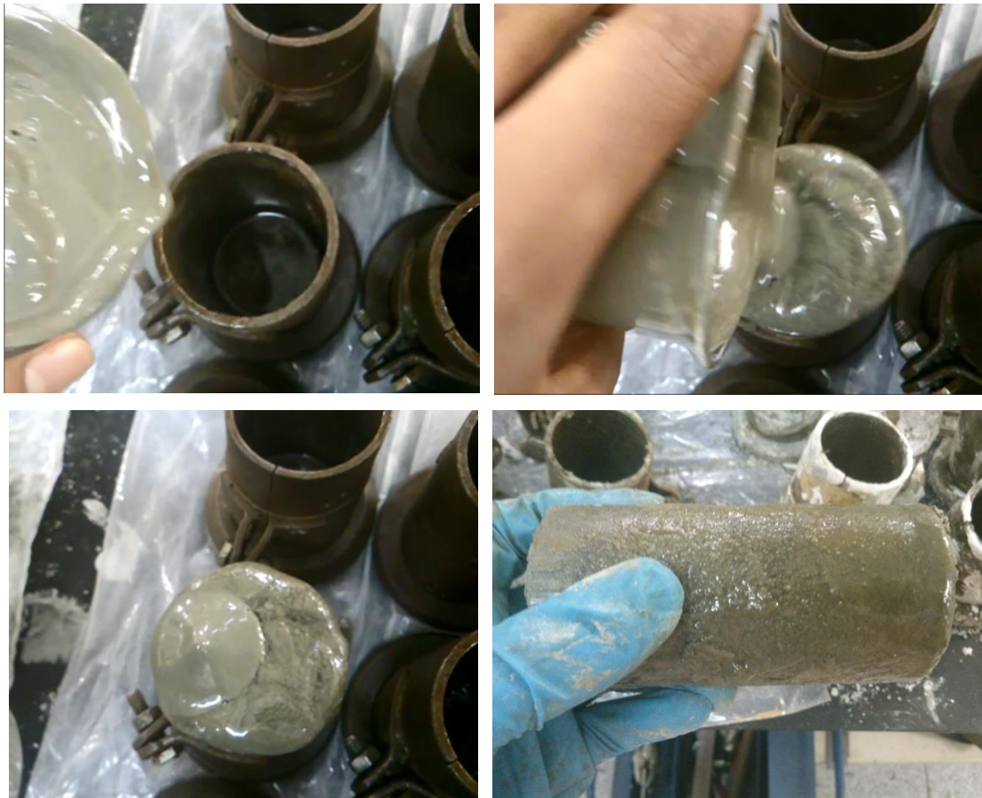
Figure 7.14 Moulding and unmoulding of A30 grout.
