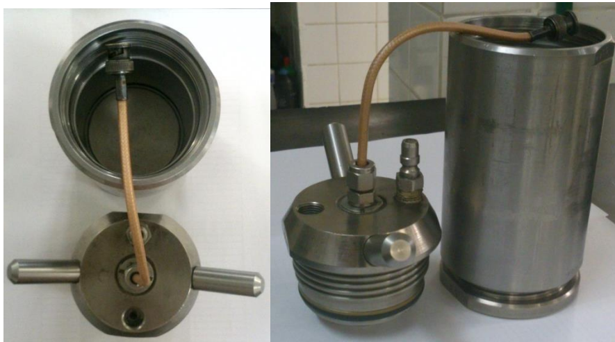
Figure 4.17 Cylindrical cell where the grout specimen is poured
