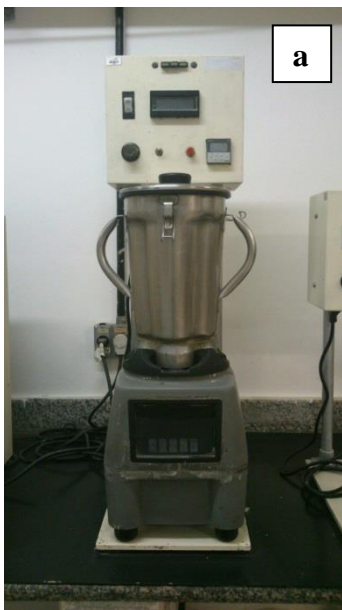
Figure 4.13 Chandler Engineering mixers a) whole view; b) propeller
