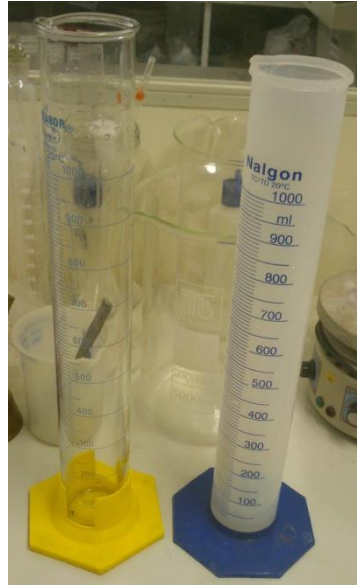
Figure 4.21 Apparatus used for the Expansion and Bleeding test for Grouts
