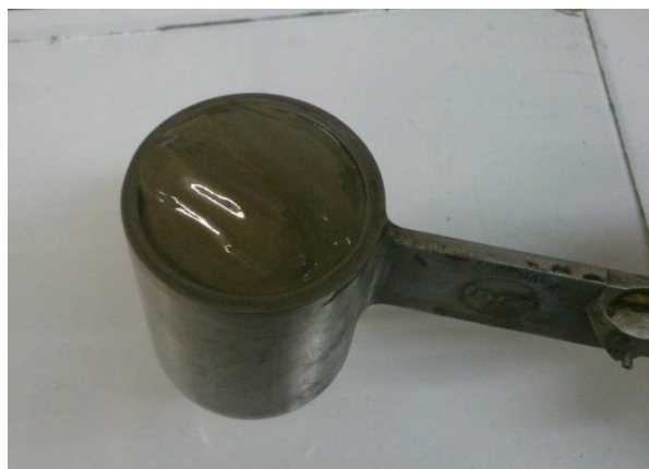
Figure 6.3 CBFA grout sample before test
