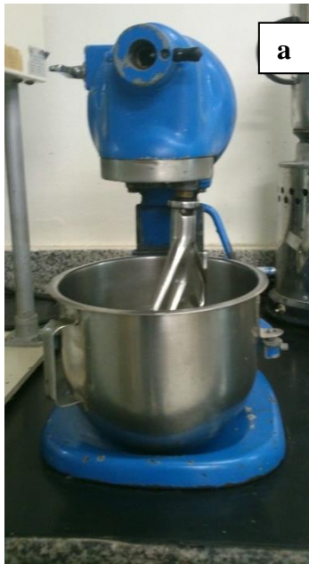
Figure 4.12 Hobart planetary mixer: a) whole view; b) “B” flat beater
