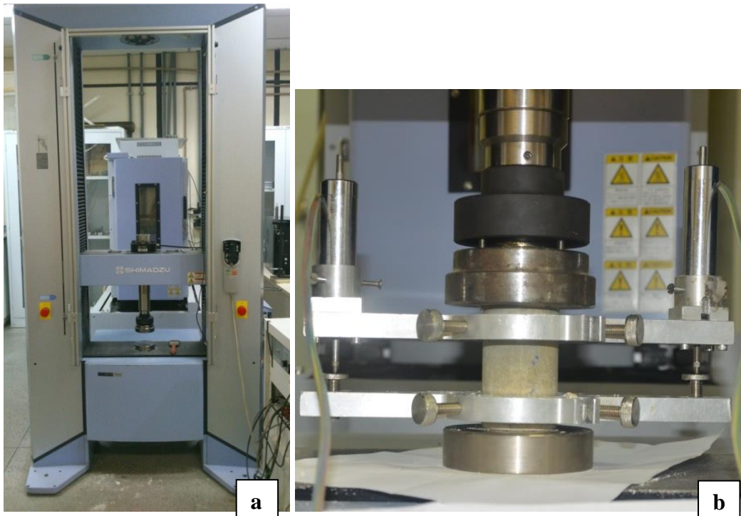
Figure 4.22 Compression test equipment a) Shimadzu AGX-100 kN testing machine, b) LVDTs arrangement b)
