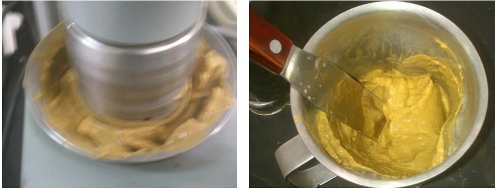
Figure 5.6 Highly thixotropic behavior of 10% bentonite suspension
