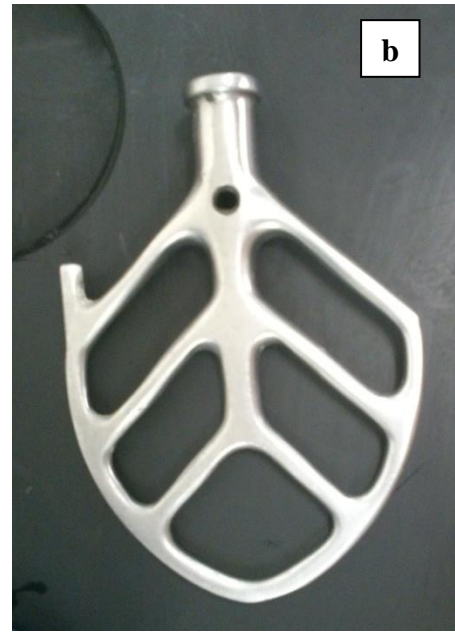
Figure 4.12 Hobart planetary mixer: a) whole view; b) “B” flat beater
