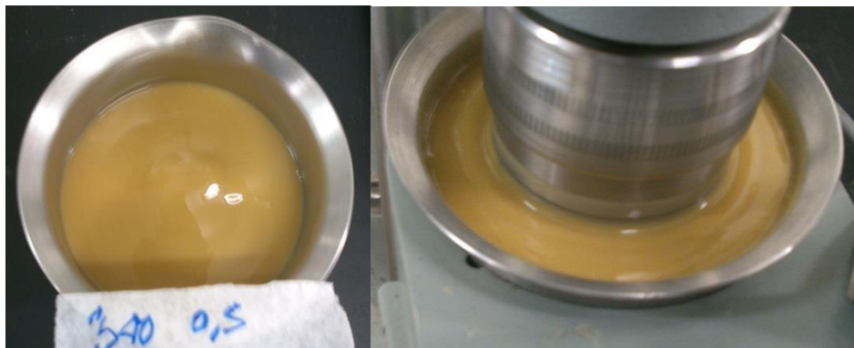
Figure 5.3 B40 or 4.58% bentonite suspension
