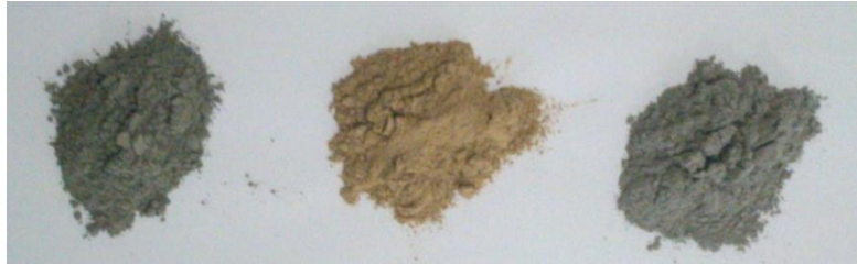
Figure 3.1 CII F-32 Portland cement, sodium activated bentonite and fly ash
