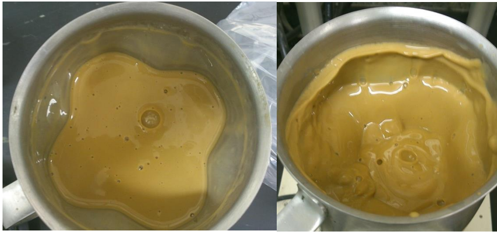
Figure 5.8 Appearance of bubbles after mixing.
