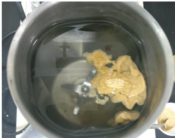
Figure 5.1 Importance of proper dispersion of bentonite.
