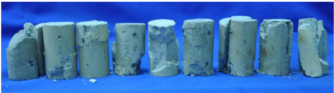
Figure 6.21 Mechanical compression of CB40FAx specimens at 92 days
